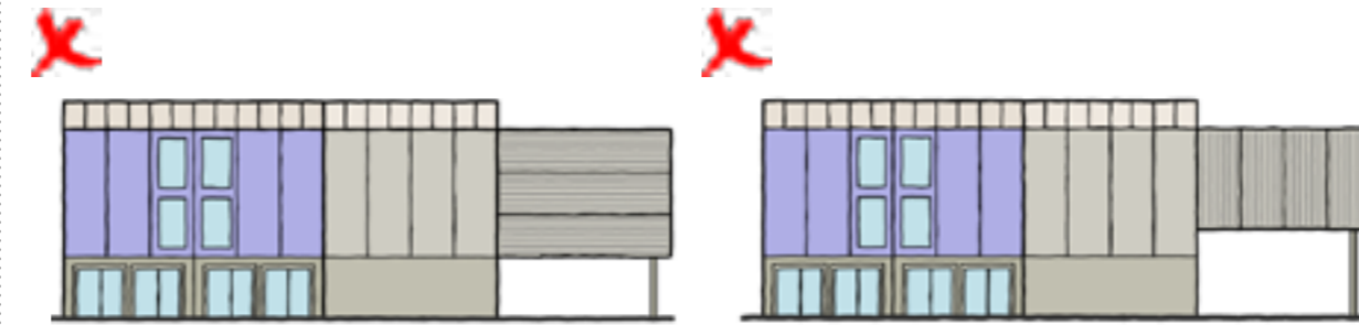
E.g. plant gantry screening design does not follow structural expression of main building.
