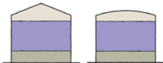
E.g. expressing building base, mid, and crown in buildings over 20m high
